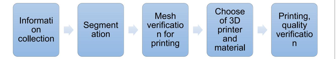
Printing, quality verification, and further steps like simulations, tests assembling, and experimental testing.
