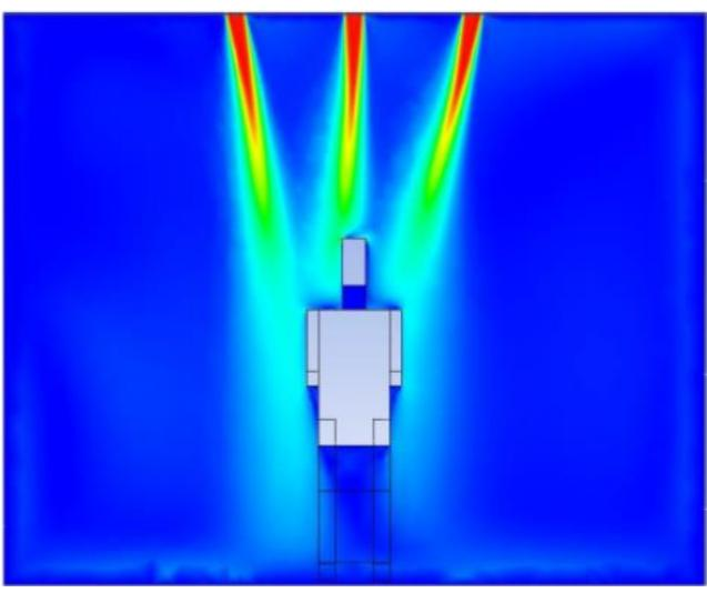
Three impinging jets with an inlet velocity of 2 m/s and the diameter of 8 cm were enough to achieve comfort regardless of the directed angle.
